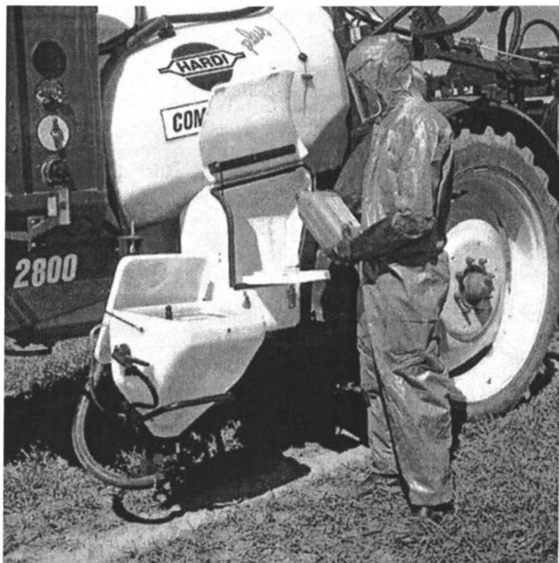
Fig 1: Operators can load sprayers quickly and safely using facilities such as this induction bowl with its container cleaning facility, PPP store and work area
